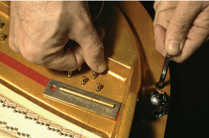
Photo 4 — Plate Height and Downbearing Adjustment
